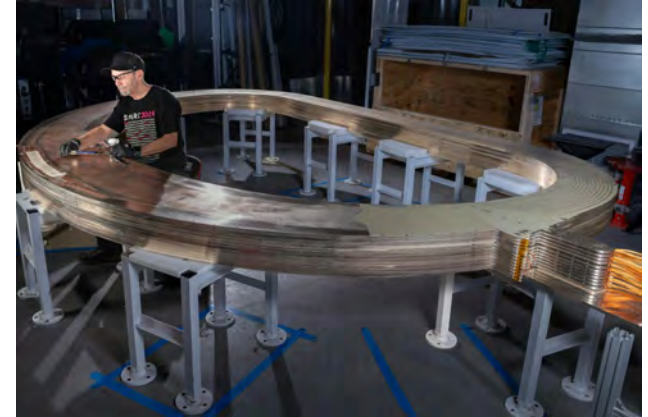
REBCO based coil at Commonwealth fusion systems
