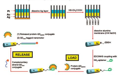
Loading/releasing of protein cargo linked nanomotor
