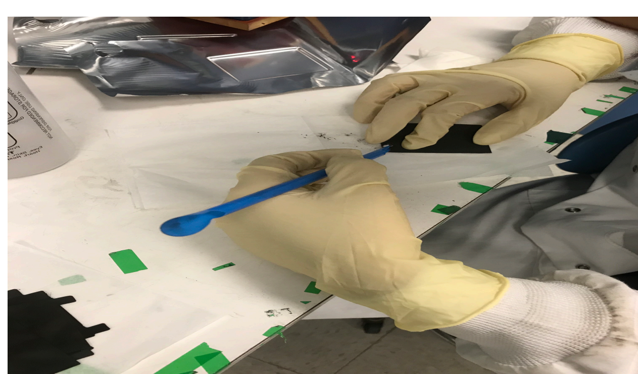
Scrapped graphite and NMC off tabs to allow for electrical connection
