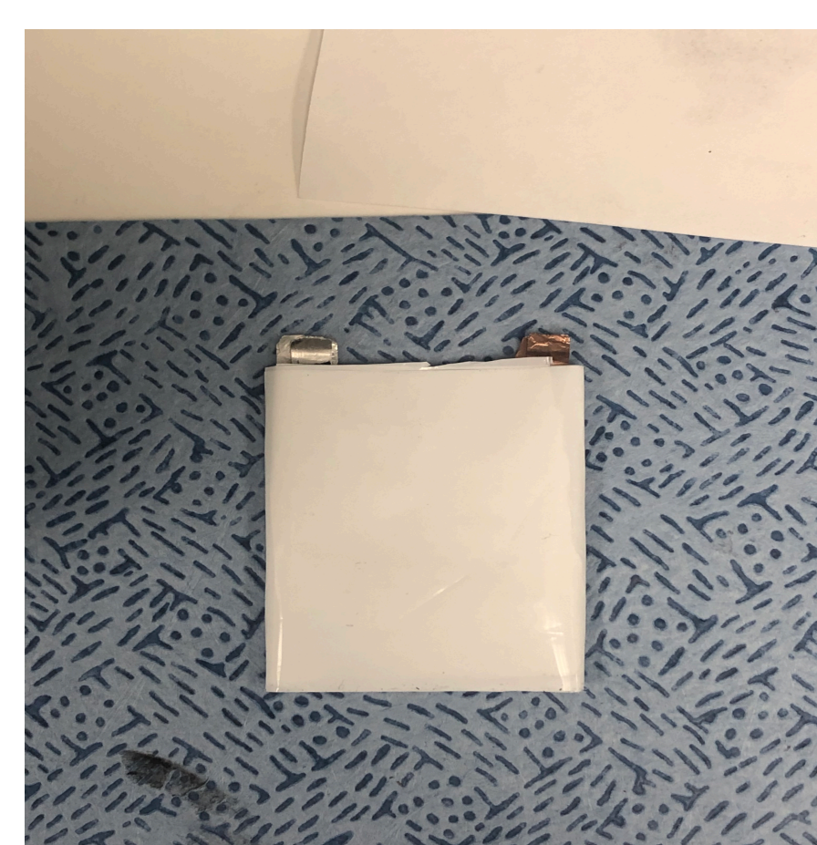
Stacked anodes and cathodes with polymer separator in between
