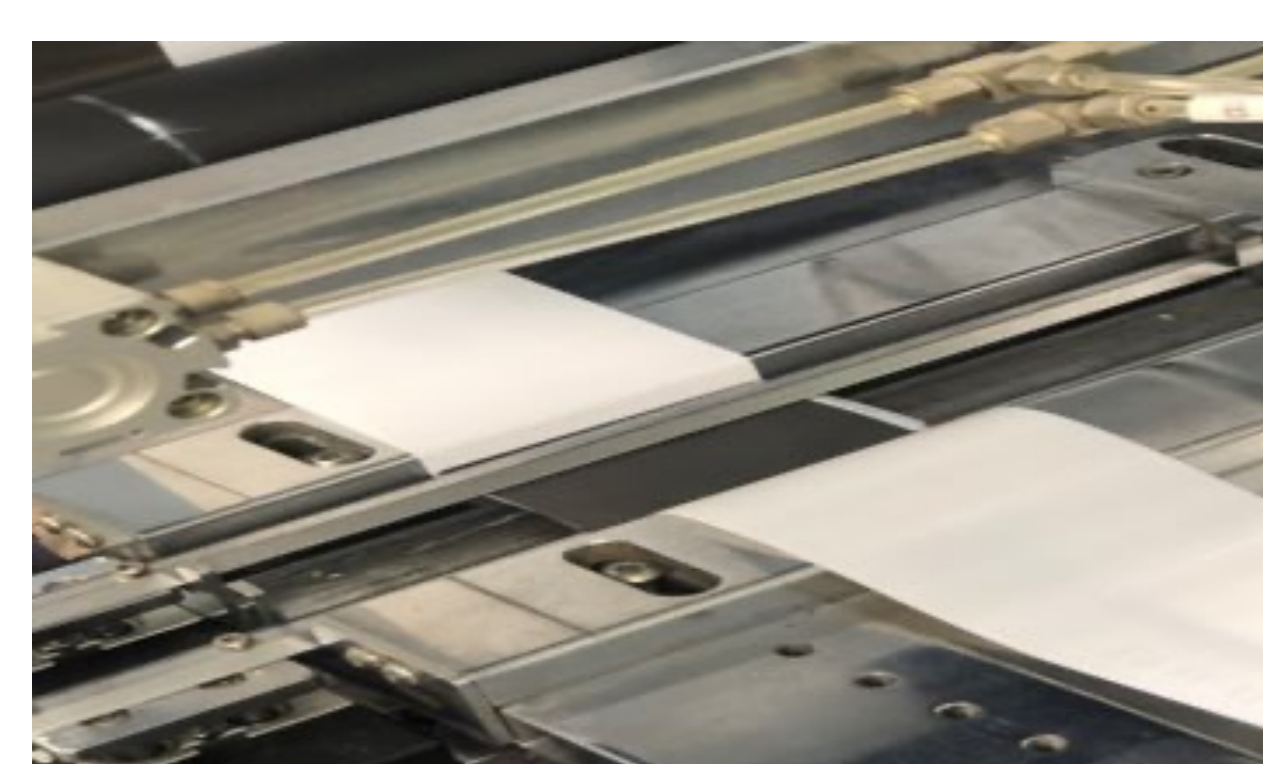
Stacked anodes and cathodes with polymer separator in between
