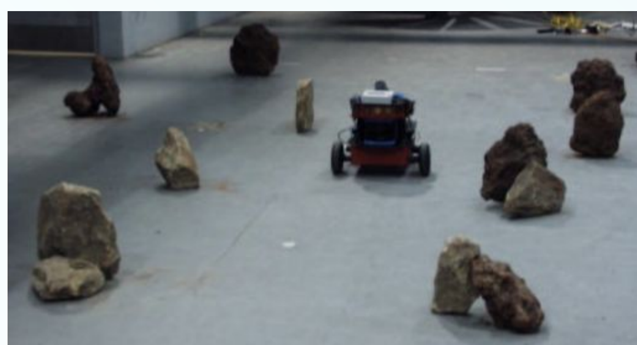
Fig 1.1 Physical robot mapping rocks, in a testbed developed for Mars Rover research, using SLAM algos
