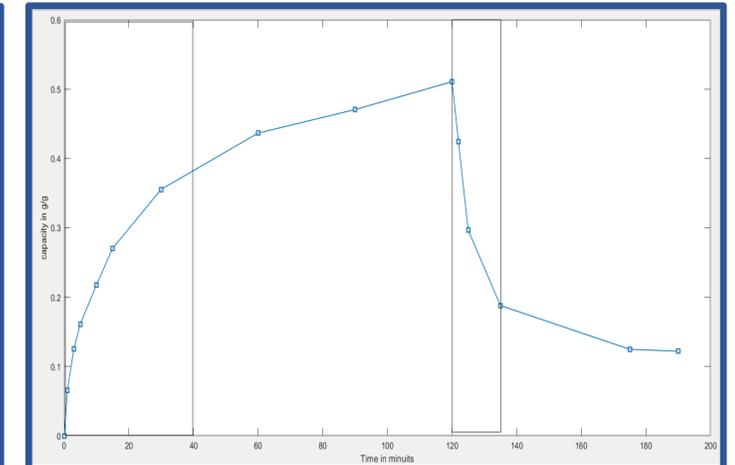
Figure 5: The absorption process follows a radical curve, while the desorption process follows a negative quadratic curve in a sudden decrease
