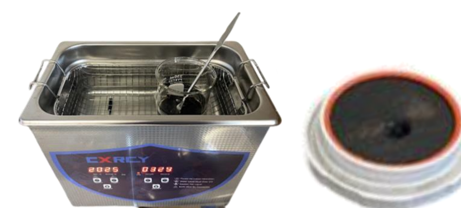
Fig. 5 Bath sonication (left) that is used to re-disperse filter cake (right)
