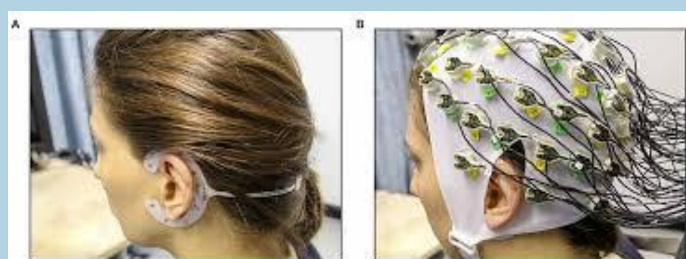
Figure 3. The application process for an ear-centered EEG compared to the traditional cap-EEG. [1]
