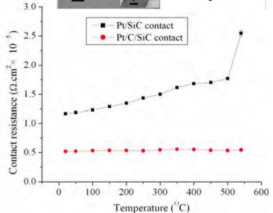
Contact resistance ( $R_c$ ) from room temperature to 550°C for Pt/3C-SiC and Pt/C/3C-SiC
