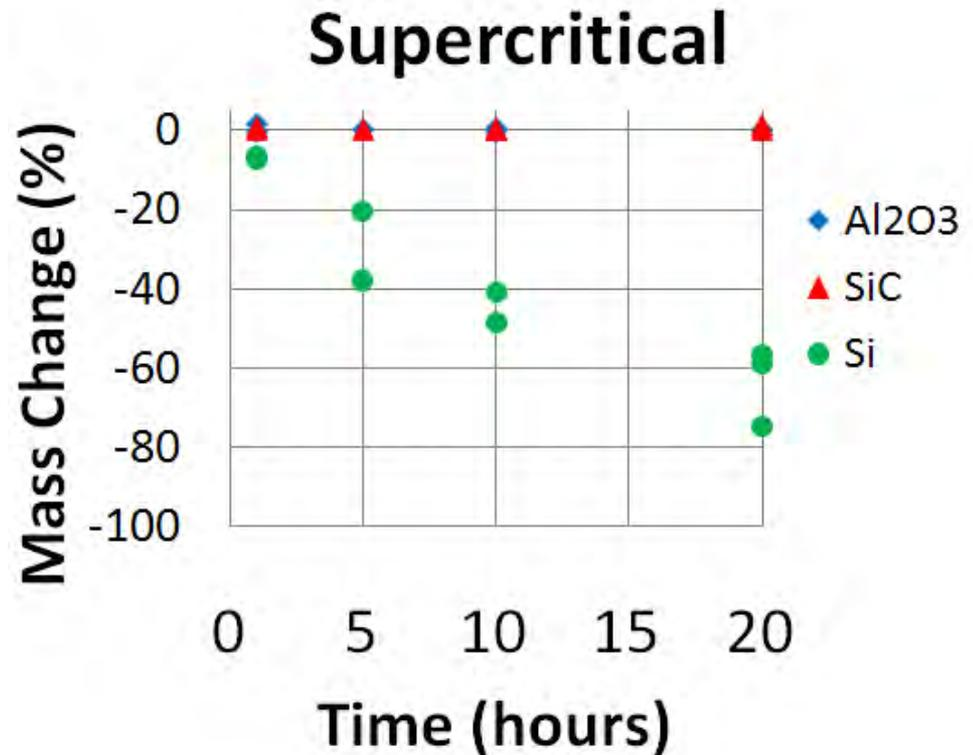
Exposure testing of sensor materials in supercritical H<sub>2</sub>O (with Ni ions) environments (P = 100 MPa, Temperature = 427°C) with Tuttle pressure vessel.
