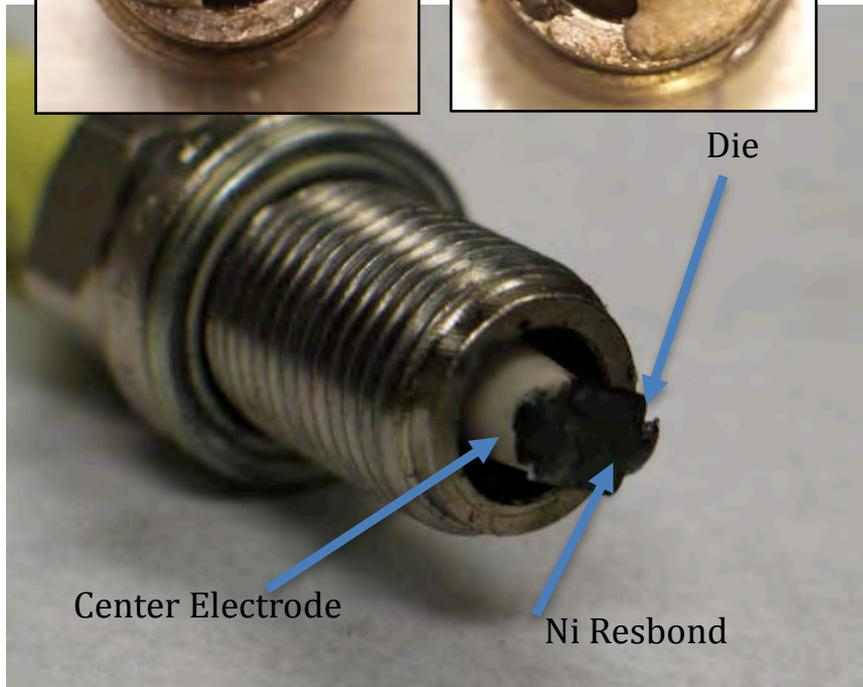
Test Fixture for signal collection. There are two die attachment methods:
