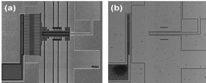
Optical images of (a) SiC-coated and (b) uncoated polysilicon structures following immersion in 65°C KOH for 1 minute
