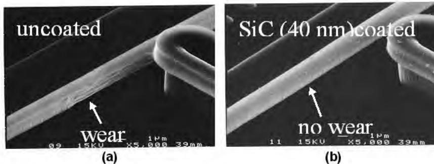
SEM images of (a) poly-Si after 250,000 cycles and (b) SiC-coated beam after 1 million cycles of high contact pressure rubbing.
