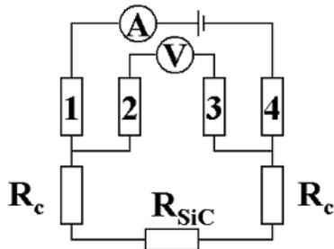
Schematics of the Circular Transmission Line Method (CTLM) structure.
