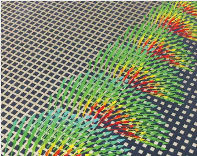
Figure: "Line waves" are confined to the infinitesimal boundary between two impedance surfaces. They have the unusual property that a forward-propagating mode is not easily scattered backward due to the symmetry of the surfaces.
