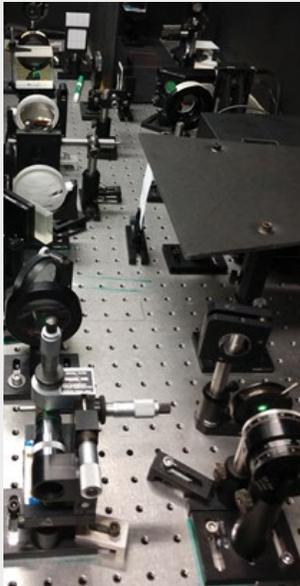
SRIP 2018 Test 1. Optical set up to produce the Gaussian spot in the picture below.
