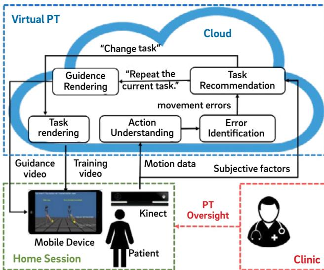
Figure: Architecture of the proposed remote training system.
