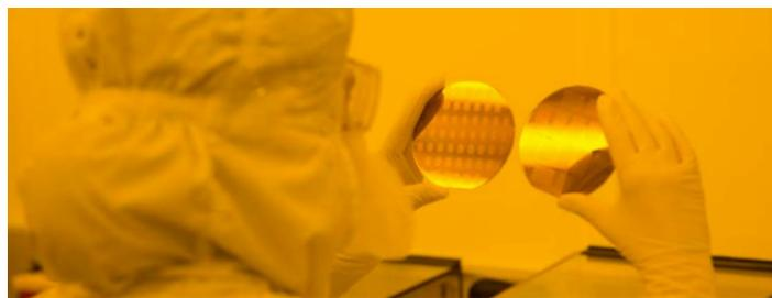
Inspecting silicon wafers used to manufacture Professor Todd Coleman's bio-sensors
