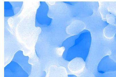
Nanofoams made from porous silica, with an average pore size of a few microns, seen at the 50-micron, 20-micron and 5-micron scale. Engineers are developing nanofoams that disperse the force of an impact over a wider area than conventional foams.
