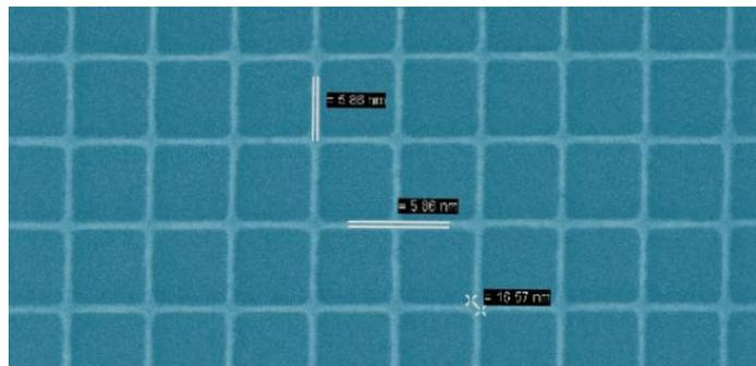
Colorized micrograph of an electron beam-written grid pattern demonstrating < 8 nm resolution capabilities of the EBPG5200.
