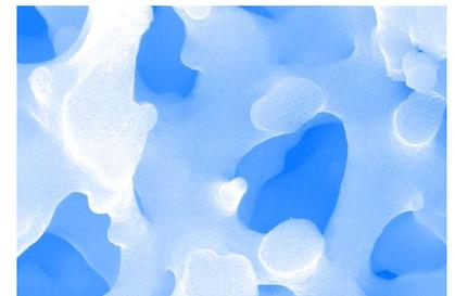
Nanofoams made from porous silica, with an average pore size of a few microns, seen at the 50-micron, 20-micron and 5-micron scale. Engineers are developing nanofoams that disperse the force of an impact over a wider area than conventional foams.
